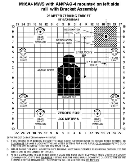
Figure G-6. 10-meter boresight target/25-meter zeroing target offsets.
